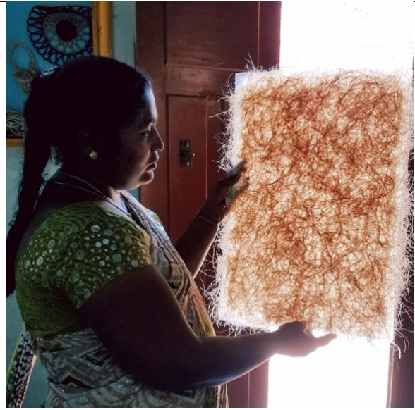
Composite sheet after heating & pressing
