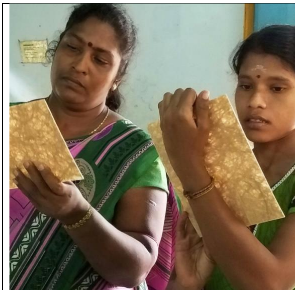
Multiple composite sheets pressed together and cut to size
