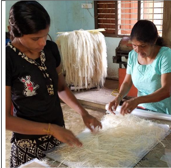
Banana fiber layered between plastic
